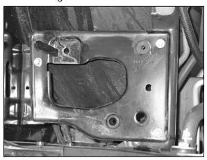
12b. Remove the heat shield assembly and drill a 5/8" hole through the marked location from step #12a.
