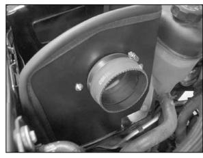
16. Install the silicone hose (08618) onto the filter adapter and secure with the provided hose clamp.
