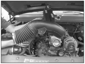
6. Loosen the hose clamps, which secure the stock intake tube to the throttle body and mass air sensor and then remove the intake tube from the vehicle.
