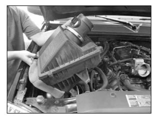
7. Pull firmly upwards to release the air cleaner assembly from the mounting tray grommets, and then remove the assembly as shown.
