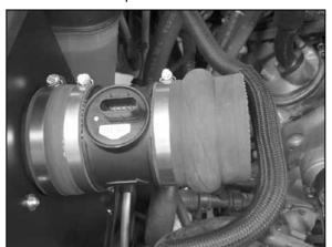
19. Install the silicone hump hose (08176) onto the K&N® intake tube and secure with the provided hose clamp as shown.
