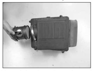
8. Loosen the hose clamp and remove the mass air sensor from the air cleaner as shown.
